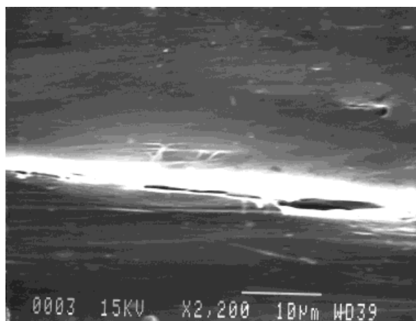
Figure 3 SEM image of the interface between ethylene-vinyl alcohol and commercial PP.
